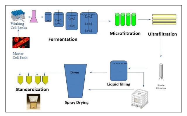
Figure 1: Schematic representation of the production process for xylanase
